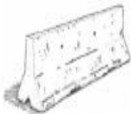
Concrete Jersey Barrier
