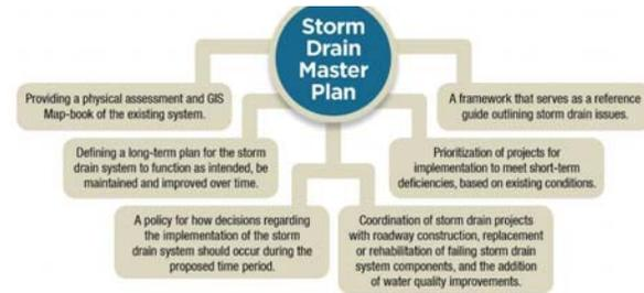
**Description:** Preparation of a storm drain master plan will provide an analysis of the existing collection system. The plan will identify system deficiencies related to capacity, functionality, and permit compliance. The plan can serve to guide future budget allocations for improvements to the system.
