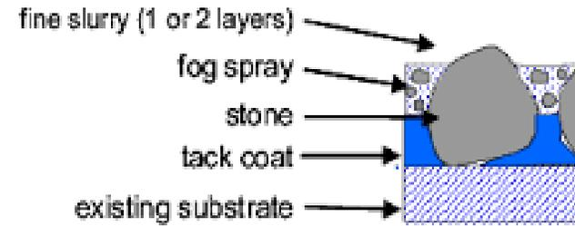
**Description:** Based on the most current P-TAP report, various pavement segments will benefit from a cape seal. A cape seal is applied when a slurry seal or micro-surfacing will not adequately address the pavement deterioration. Cape seals are a multi-layered treatment pavement preservation treatment which can extend the life of a pavement by 6-8 years.
