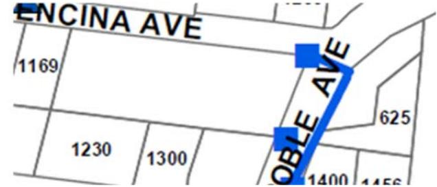
**Description:** The existing system appears to have capacity issues at Roble Ave. and Encina Ave. that warrant review and upgrade. This project will assess the collection system for capacity and hydraulic profile and upgrade the system as necessary.
