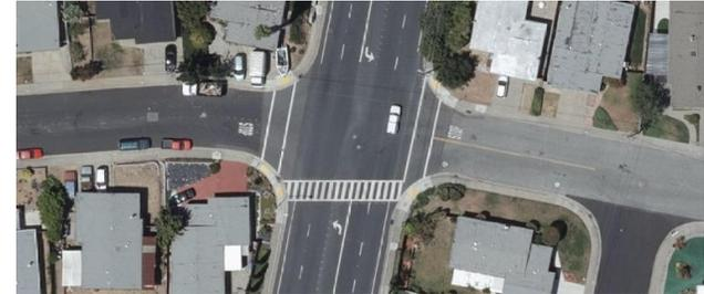
**Description:** The key elements affecting the safety of pedestrians and cyclists at the Appian Way and Marlesta Way intersection is speed and reduced visibility of approaching traffic due to the topography of the project area. Safety improvements are required to improve crossing conditions for pedestrians and bicyclists. In February 2021, the City selected a Consultant to complete the preliminary engineering for this project.
